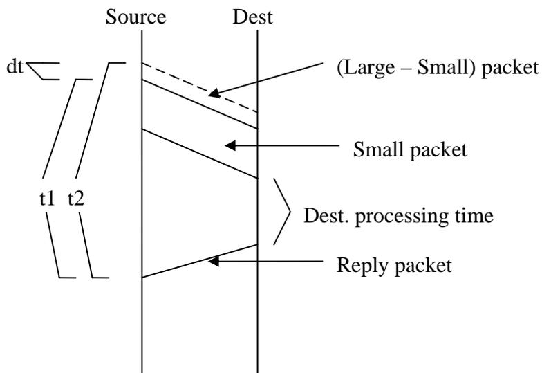
At the base of calculation lies the formula  $\text{bandwidth} = \text{datasize} / \text{transfertime}$
